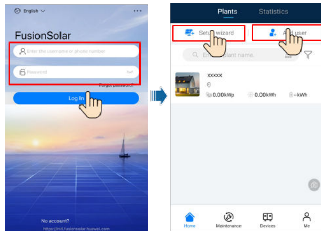
Figure 7-5 Creating a PV plant and a user
