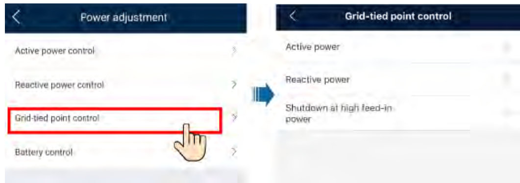
Figure 7-11 Grid-tied point control
