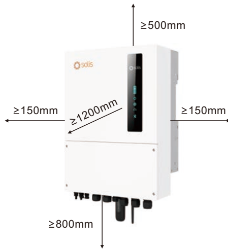
Figure 3.5 Inverter Mounting Clearances
