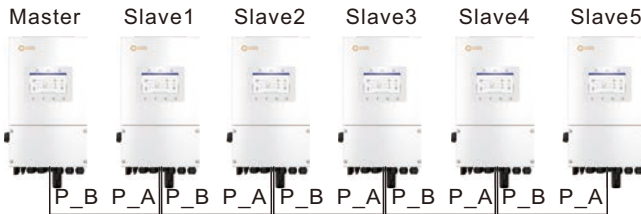
Figure 3.24 Parallel Terminal Connection
