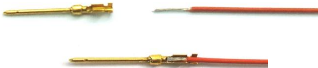
Figure 5.7 Making a communication cable
