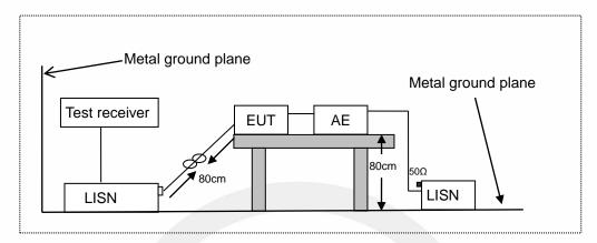
LISN: Line Impedance Stabilization Network
