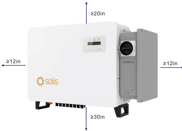
Figure 3.2 Clearance distances requirement for the inverter
